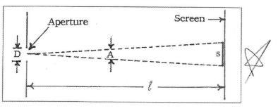
see more detail. If we want to know the *linear* size of the Airy disc, we can calculate it with the help of the diagram at the right. Let s be the diameter of the disc, defined as the diameter of the first dark circle, while  $\ell$  is the distance from the lens or pinhole to the image. Then, since A is in radians,  $A = s/\ell$  and we find that  $s = 2.44 \lambda \ell/D$ .
